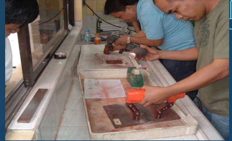
Penetrant and Magnetic Particle Testing
