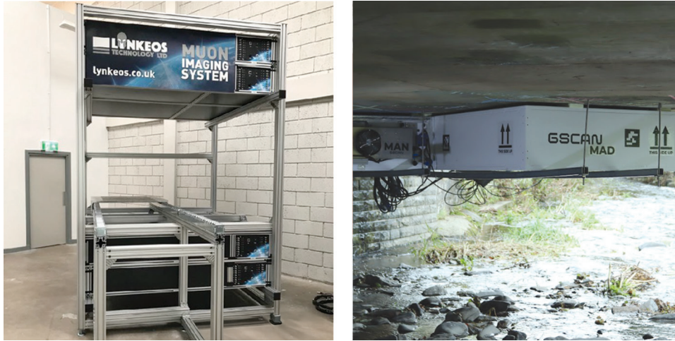
Figure 3. Examples of muon tomography detecting systems: a laboratory set-up of Lynkeos Ltd (left); and a mobile system by GScan Ltd (right)
